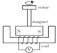
When the rotor is turned the magnet rotates, inducing a voltage in the coil. The induced voltage can be decreased by
